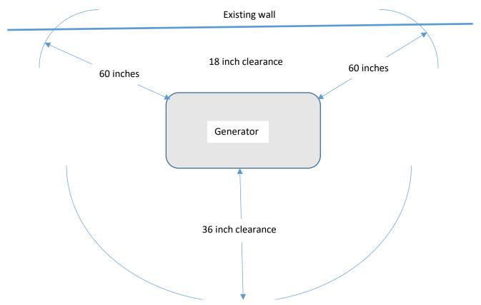
Clearance from the ends and front of the generator shall be 36 inches minimum.
